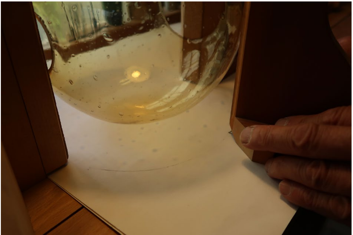
The curvature of the glass is followed by a contour tool, where the profile is transferred with a stylus to the template board. When the wooden handle is pulled across the surface, an attached pen transfers the shape of the glass to the paper.
