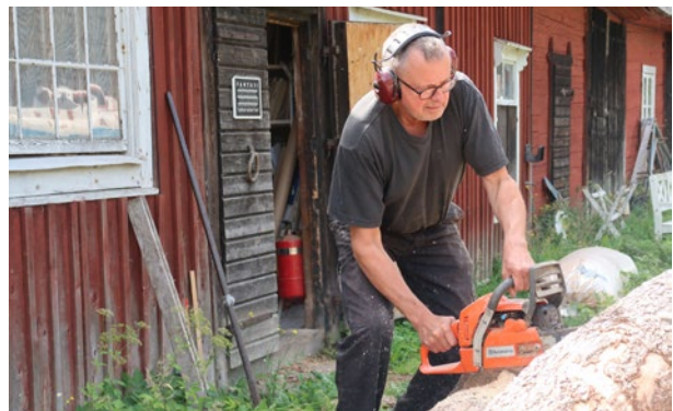
Gunnar chooses a knot free and moist part of a log, and saws out the required amount for the next shape.
