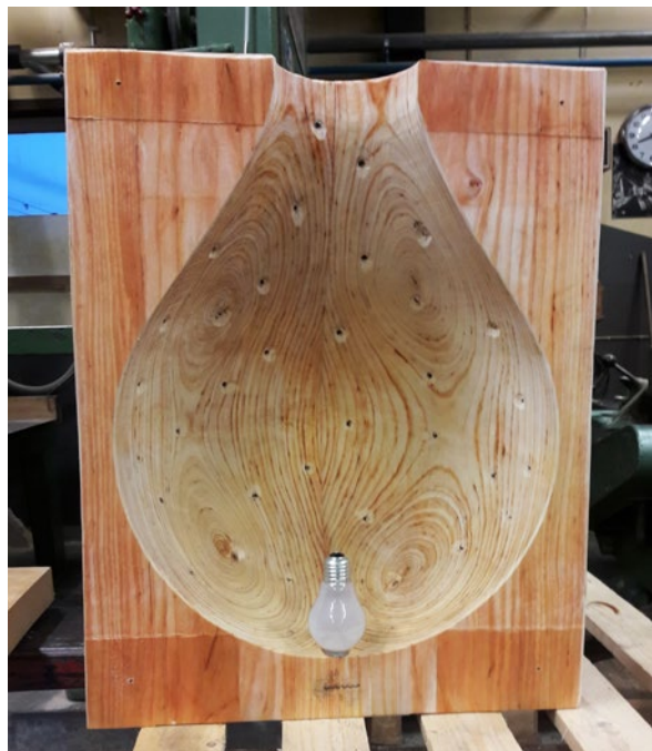
One half of the pre-cut wooden mould before mounting. The inside dimensions of the mould are a total of 600 mm high and 470 mm in diameter. Photo: Thomas Jacobsson.
