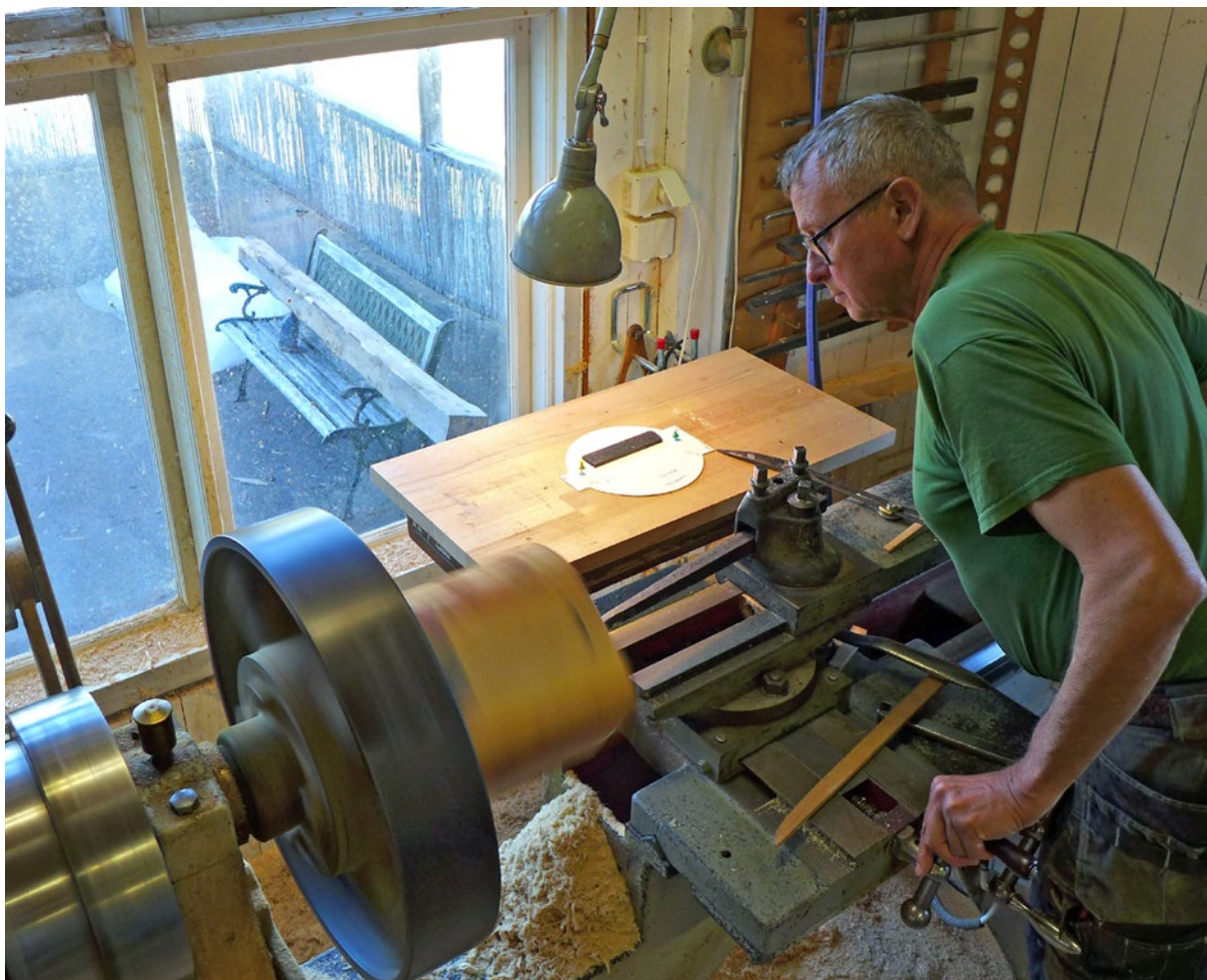
Boring is underway to achieve the internal shape, the void that is formed when the mould is finished. Photo: Andreas Flink.
