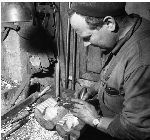
A wooden mould that has been carved out by hand is smoothed with a knife. Picture from the 1950s. The angle of the air channels indicates that the shape is a small bottle. Photo: Jan-Erik Anderbjörk, Smålands museum.
