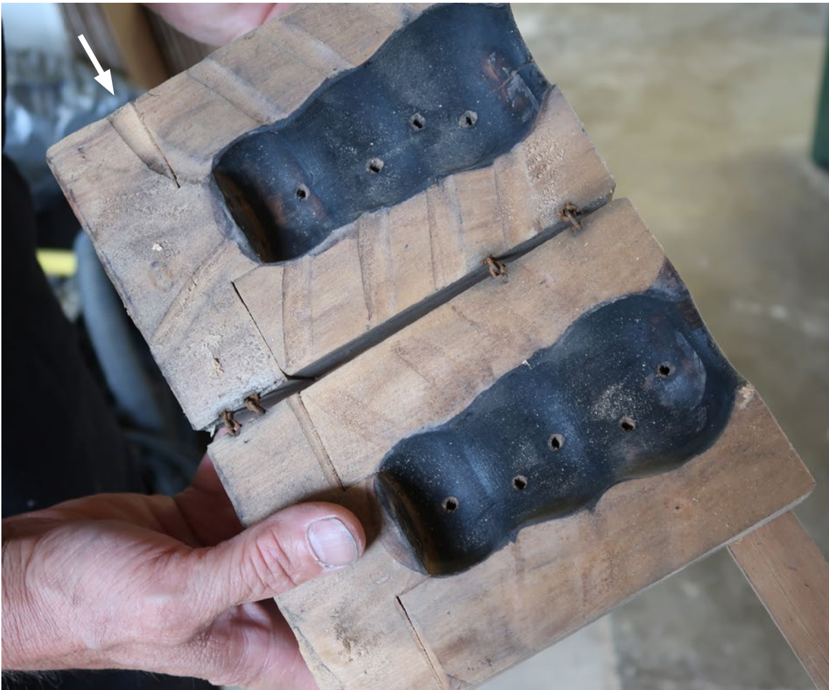
Gunnar shows a finished mould with air holes in both halves and air channels, which are made in only one half of the mould. (see arrow).
