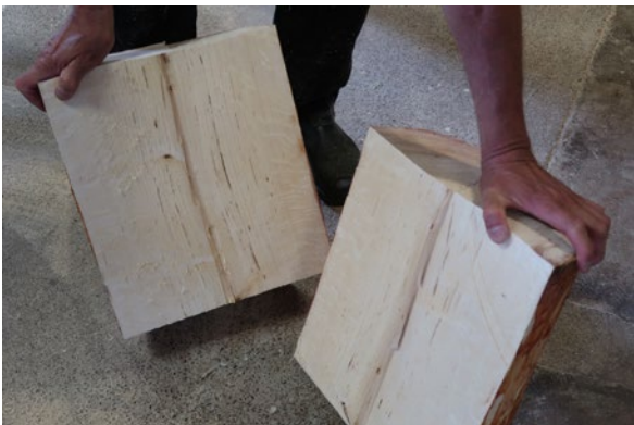
Gunnar divides the piece into two equal parts, using the circular saw.
