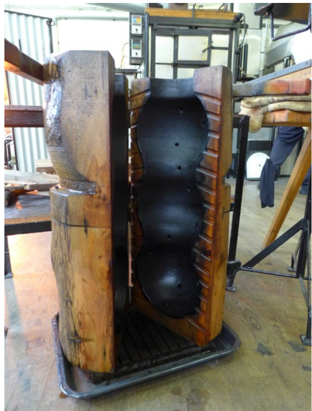
Before the wooden mould is to be used in the glass workshop, it is burnt out, i.e. one burns off the mould's surface so that it is charred and thus sealed. Photo: Gunnar Englund.
