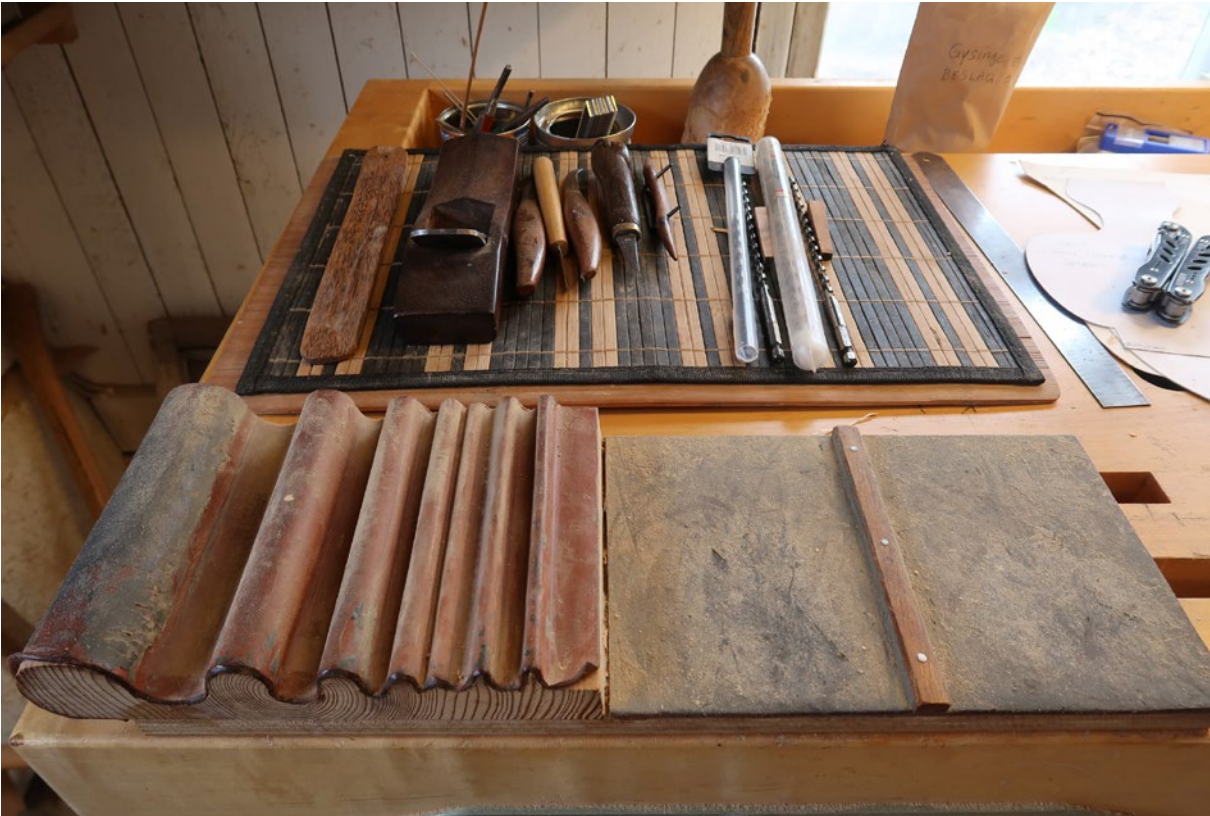
Profiled and leather-clad boards with slip paste for honing and sharpening cutting tools.
