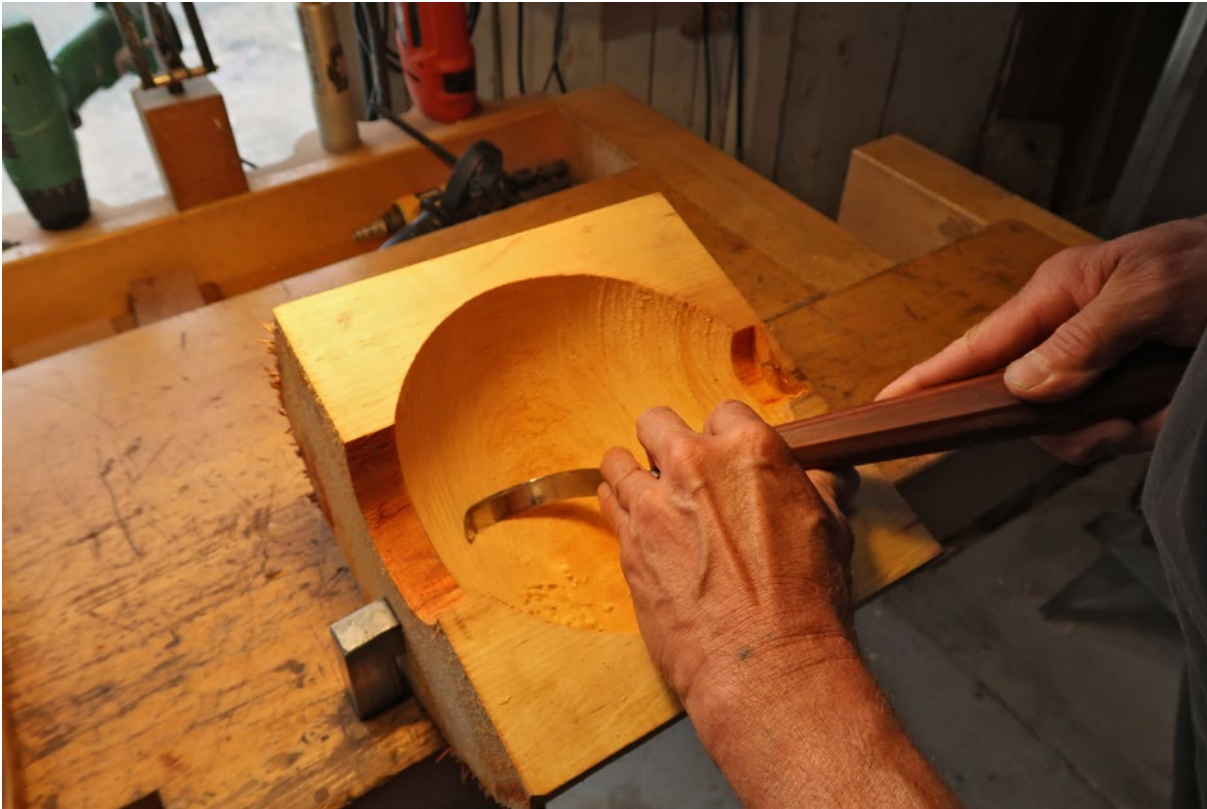
Gunnar smooths the surface with a hand-forged hook knife. The work requires patience and calm and is an important, meditative part of the profession.
