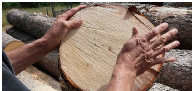
To keep track of the direction of the grain, in order to avoid knots in the mould, the top is always marked with a cross.
