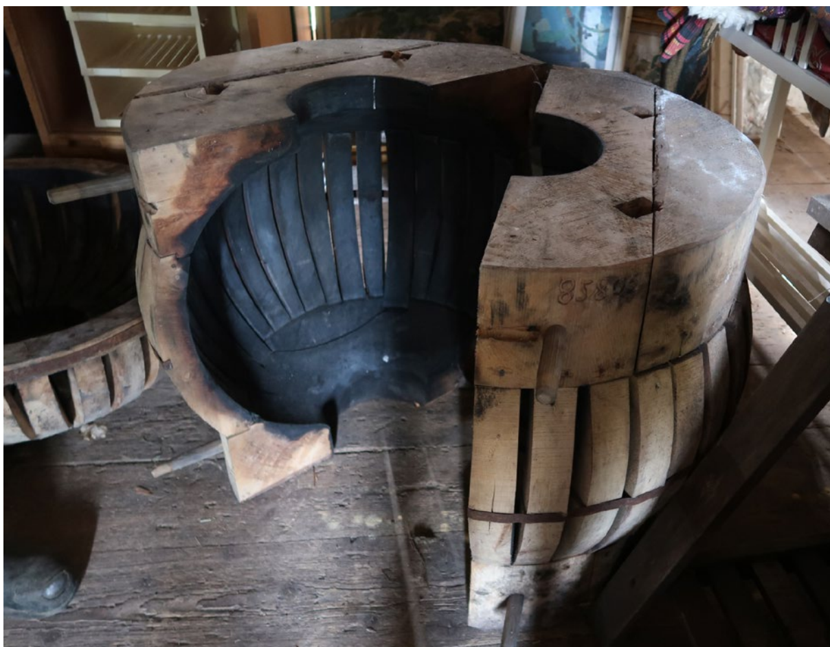
Slat or rib shapes were used in the past to blow very large glass vessels. These moulds belong to Pukeberg.
