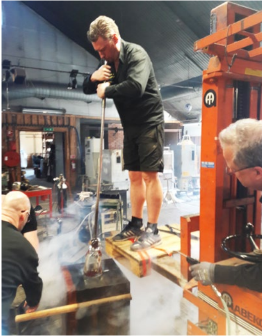
The exact mould “in action” in the glass workshop. A tough match for Lars Axelsson at Bergdala glass factory, who must have the help of the whole team to manage to blow the large piece. Among other things, being lifted (and later down) with a forklift during the process. Photo: Thomas Jacobsson.
