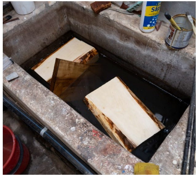
In the old milk room, a trough is used to soak moulds so that they do not crack.
