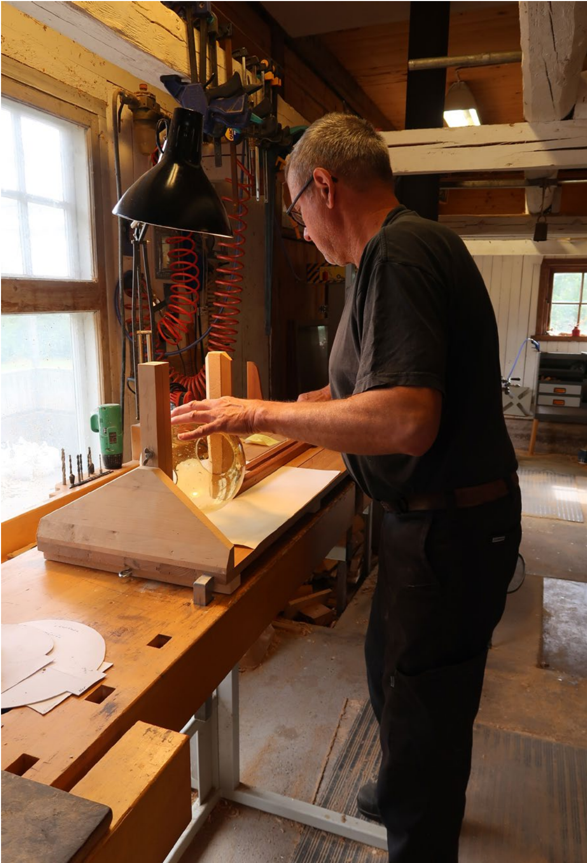
In the "Horse" the glass object is clamped firmly in order to be copied exactly.
