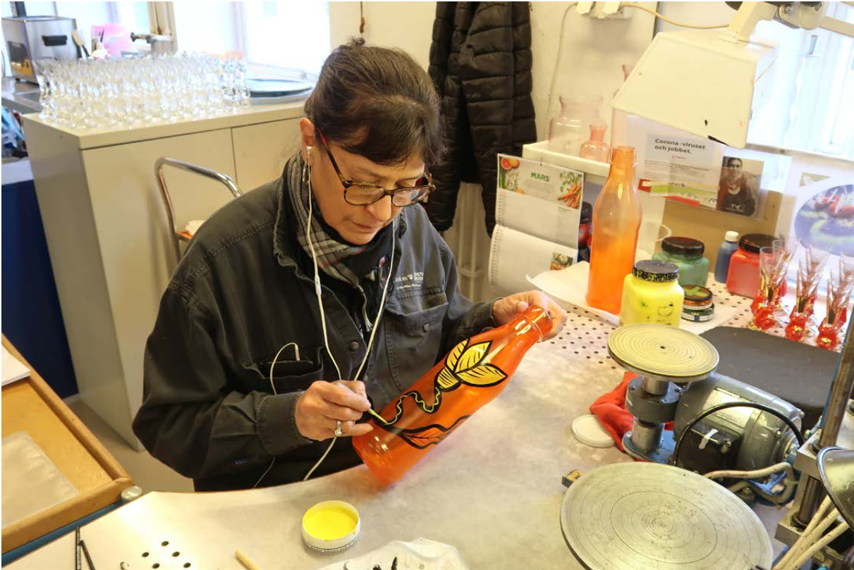
Free-hand painting with a brush. The painter holds the glass at the desired angle.
