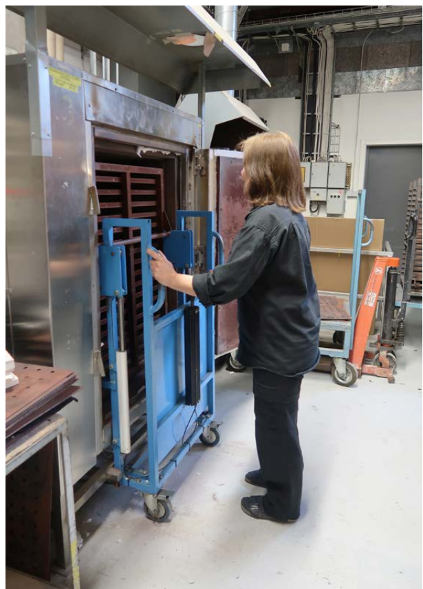
Painted glass is moved manually from the studio to the kiln – in this case by Diana Valle and Susanne Sjödin. The pictures show a kiln in Kosta, in Spring 2020, being emptied and then filled with new glass to be fired.
