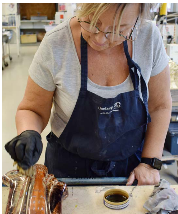
Painters at Kosta wear rubber gloves to keep paint off their hands when painting with gold. Here the paint is stippled using a natural sponge.
