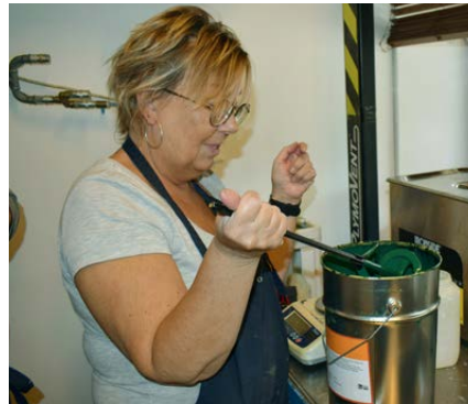
The paint is stirred with a whisk.
