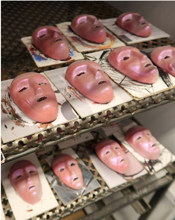
Glass sculptures by Bertil Vallien in a drying chamber before being painted a second time or being fired.
