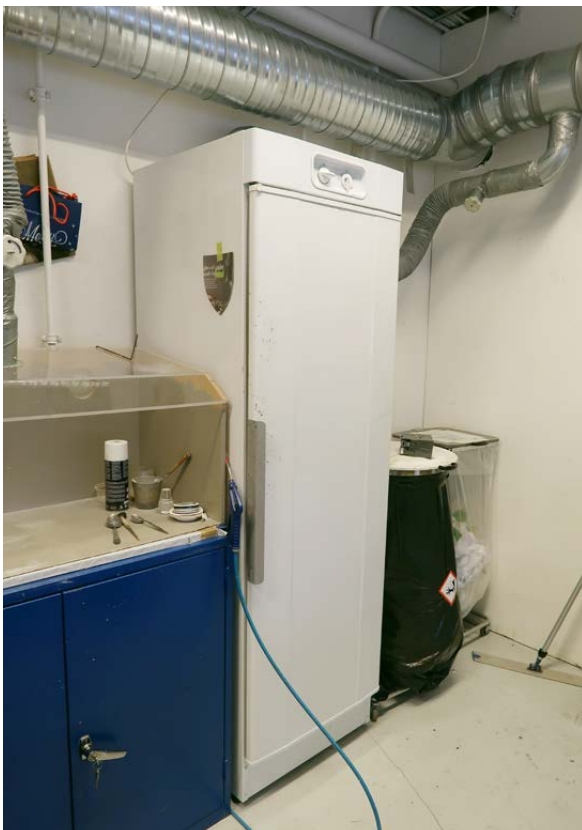
An ordinary drying cabinet will do for some steps in the process.
