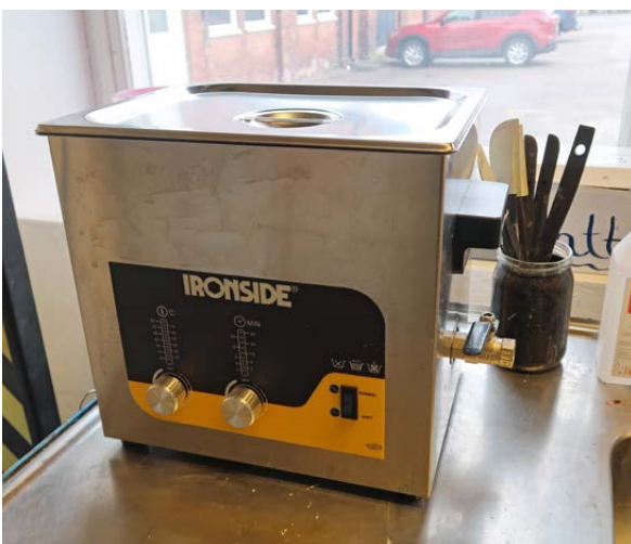
The ultrasonic washer, used to clean airbrush nozzles.
