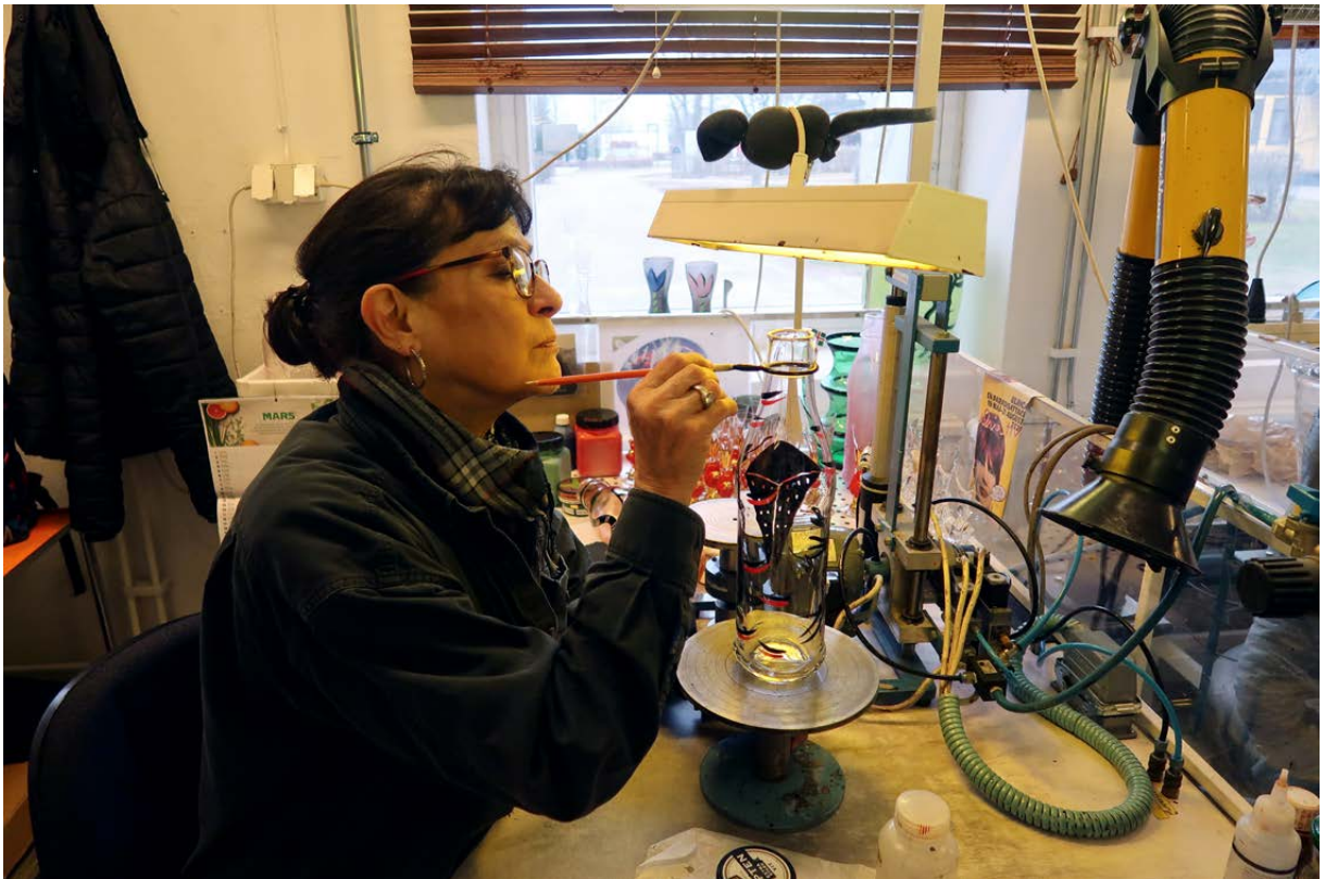
Free-hand painting with a brush. The glass stands on a cavalette that can be turned to give the painter free access to all sides of the object.
