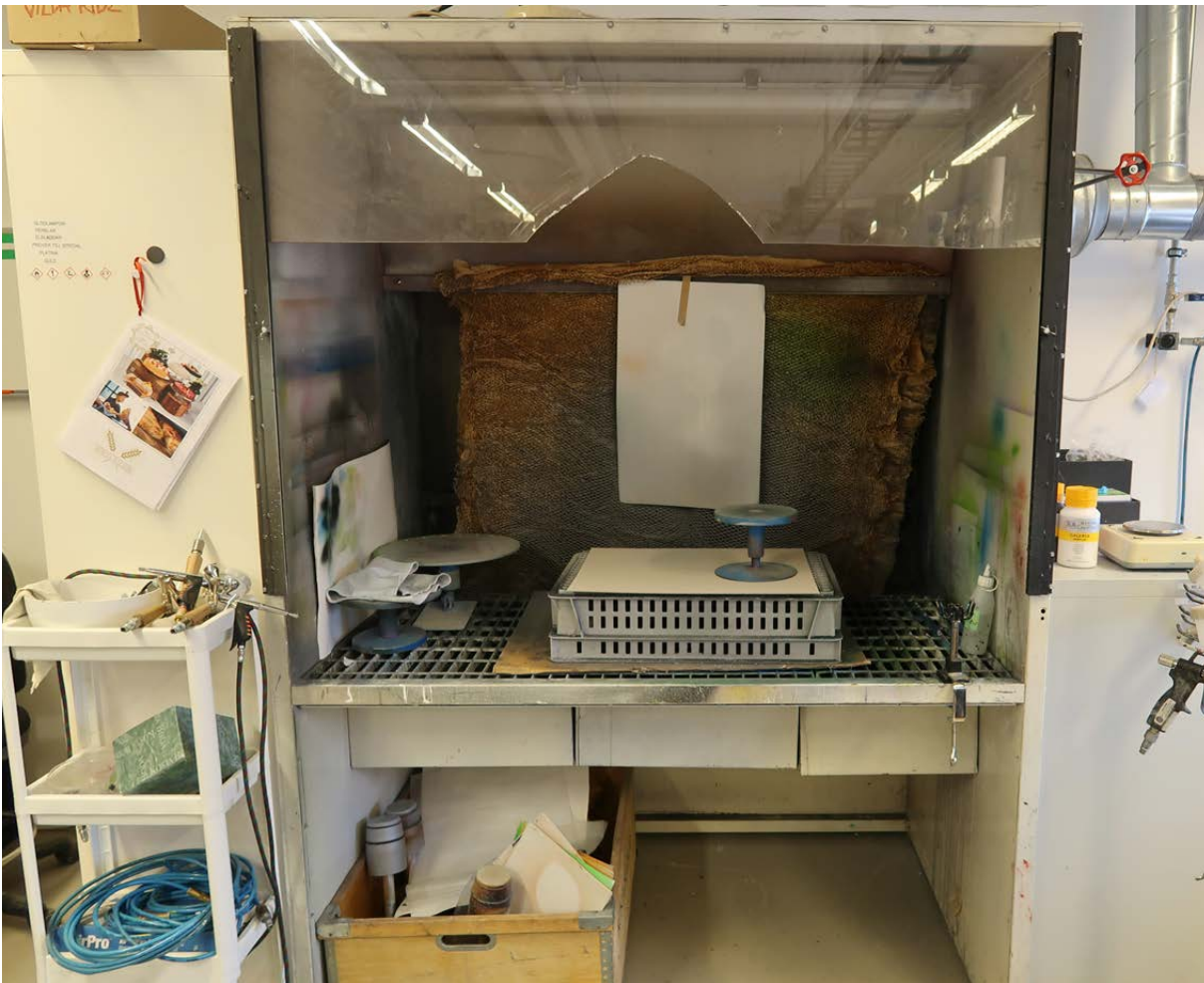
Ventilated box and airbrush equipment.
