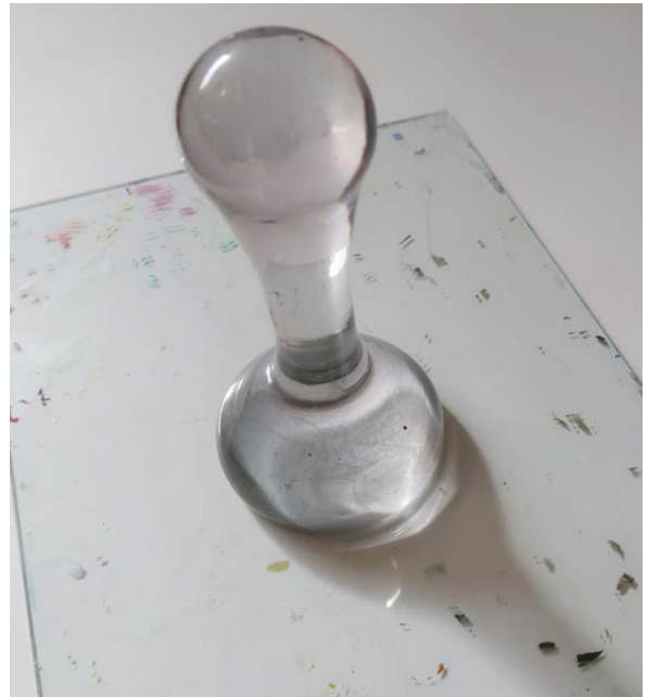
A pestle of glass was used to "bray" pigment against a flat surface, often glass. The bottom of the pestle has been 'roughed' or treated with acid; it should not be slippery. From Cecilia Almqvist's private studio.
