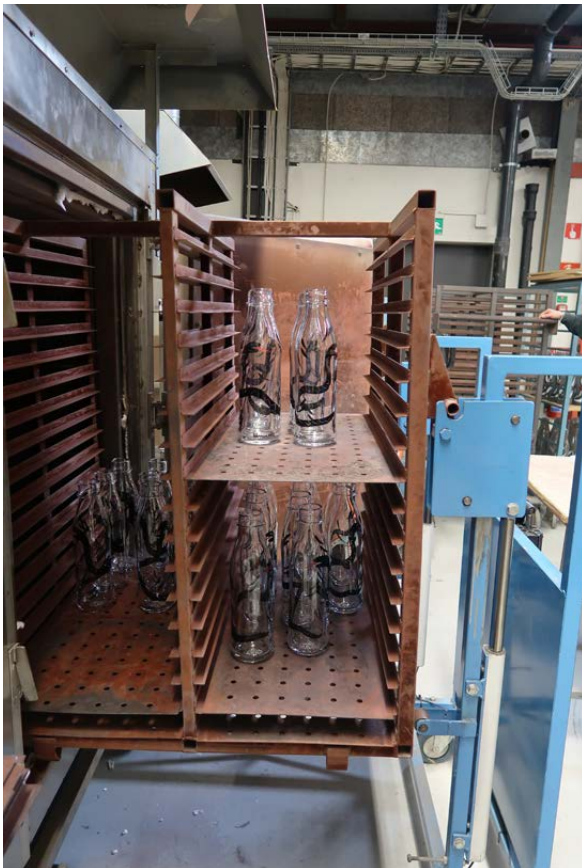
The kiln is filled with new glass to be fired.
