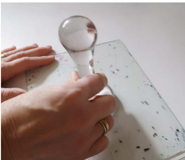
A pestle of glass was used to "bray" pigment against a flat surface, often glass. The bottom of the pestle has been 'roughed' or treated with acid; it should not be slippery. From Cecilia Almqvist's private studio.
