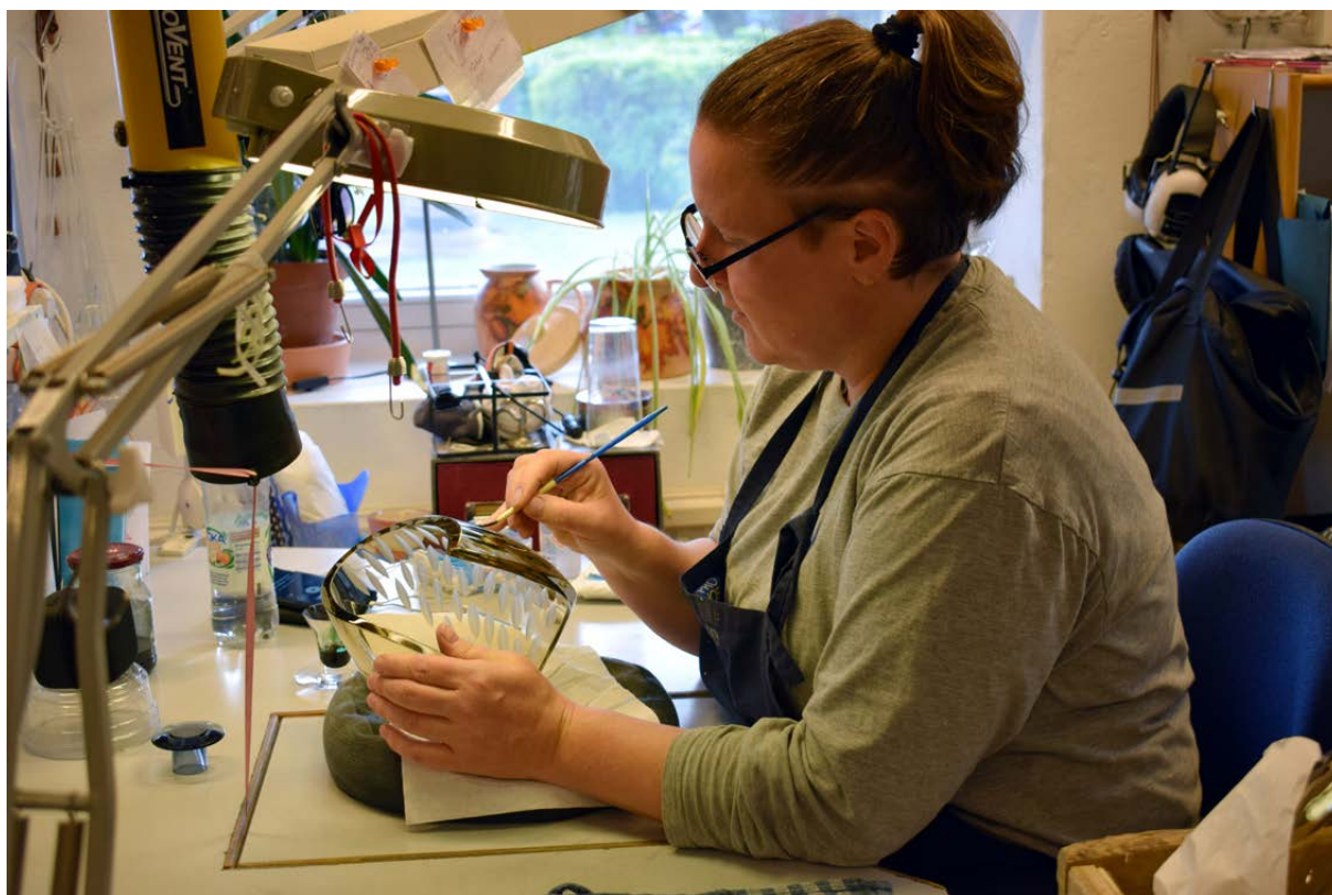
The glass has been placed on a cushion to bring it up to a comfortable height. The painter supports her elbow on the bench.
