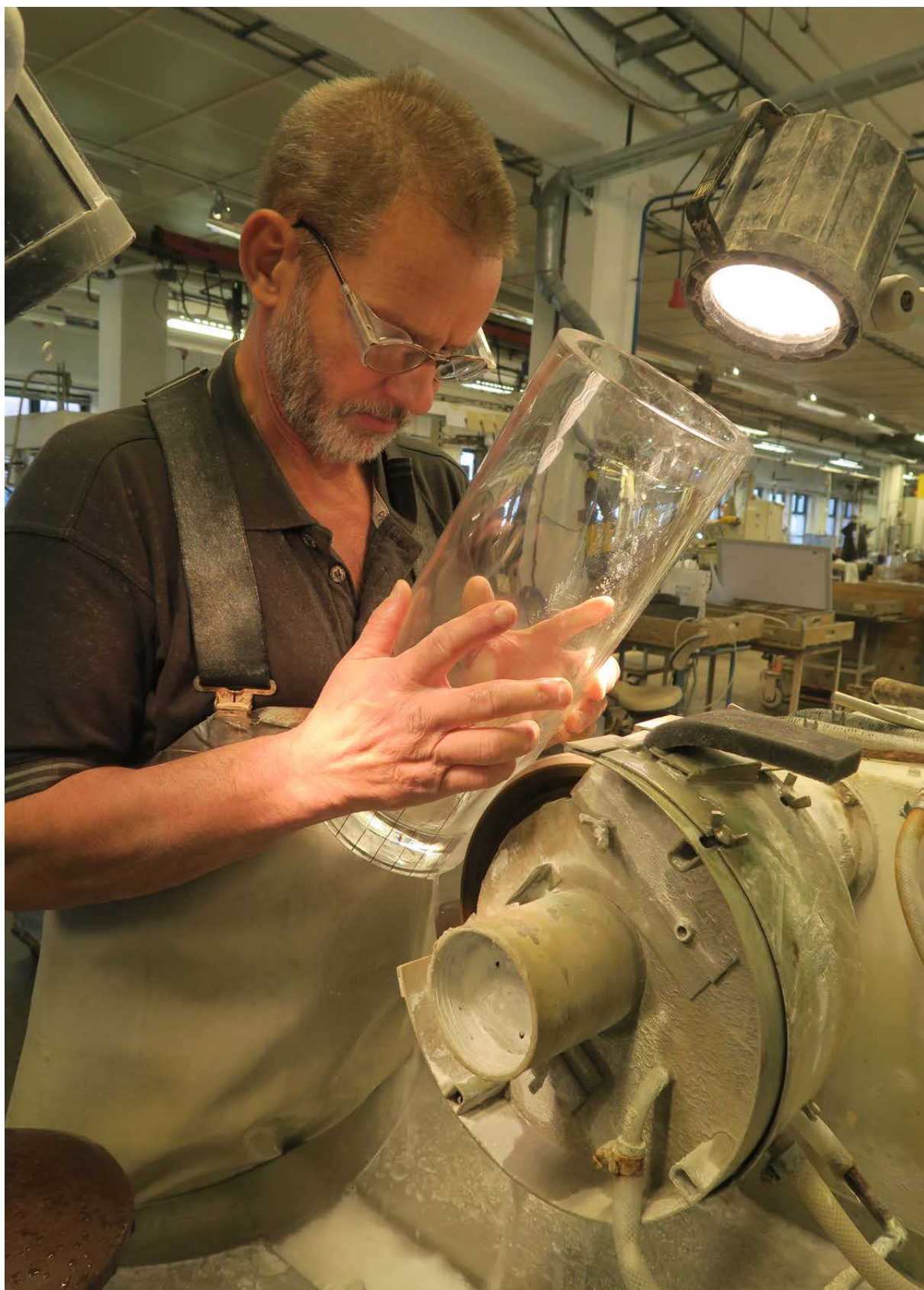
In the pictures, Anders grinds the bottom section of the vase Sarek. The step he performs in the picture is called rough grinding.
