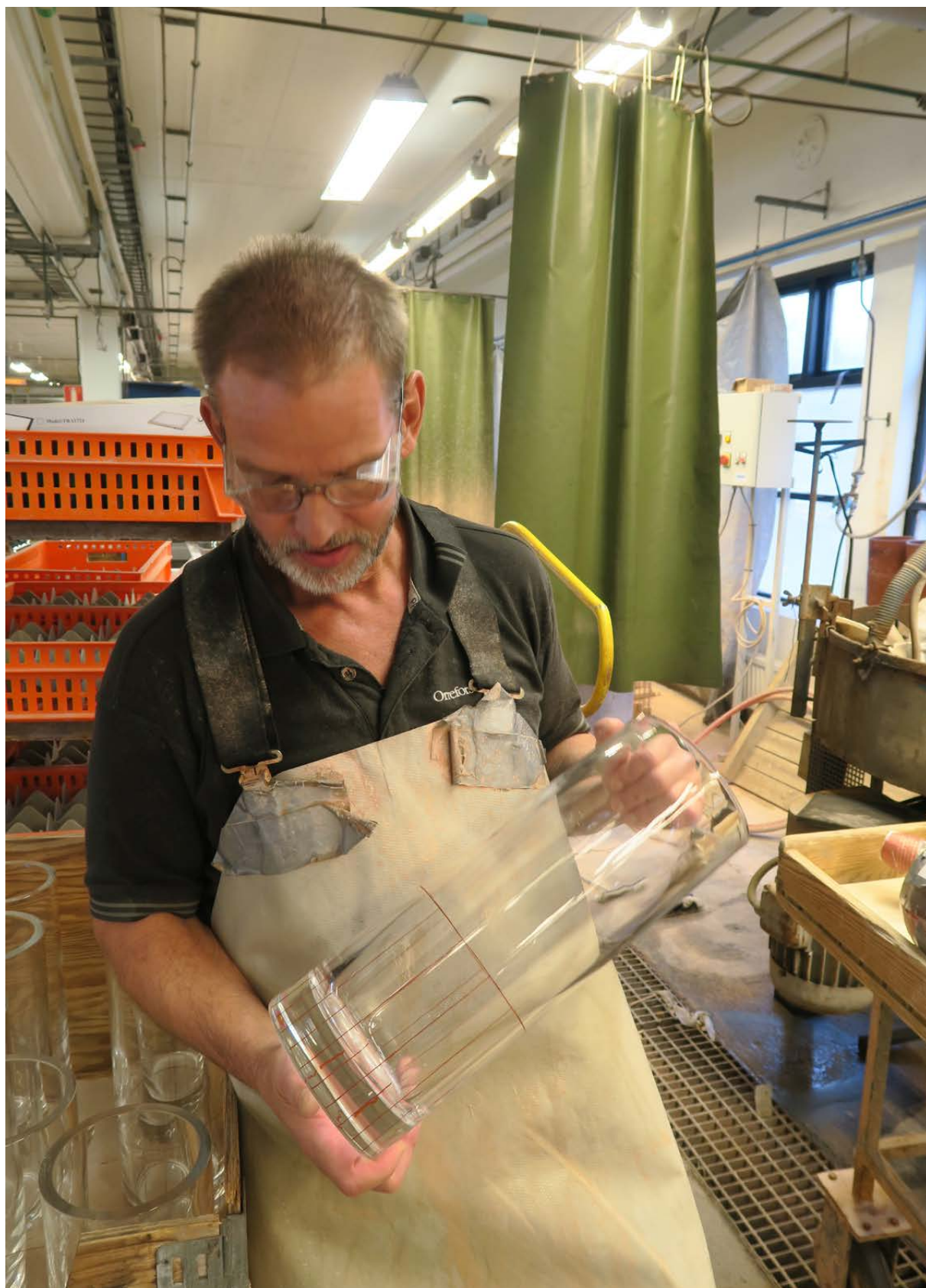
The vase has now received the desired number of lines needed for Anders to grind the vase.
