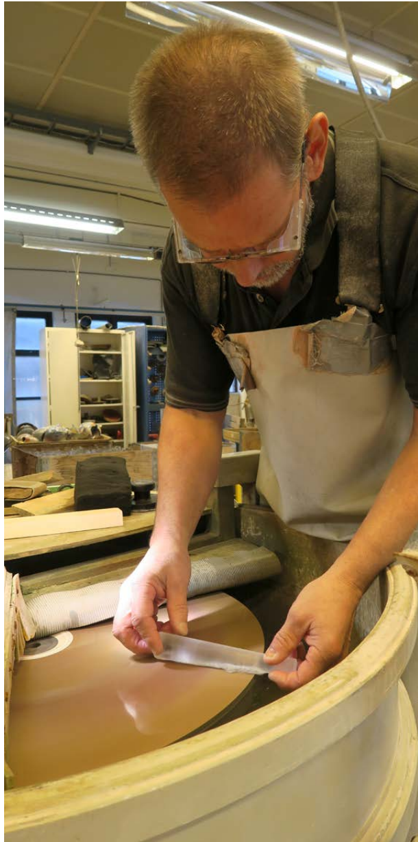
Anders here shows a type of polishing that is initially used on the glass gavel handle.
