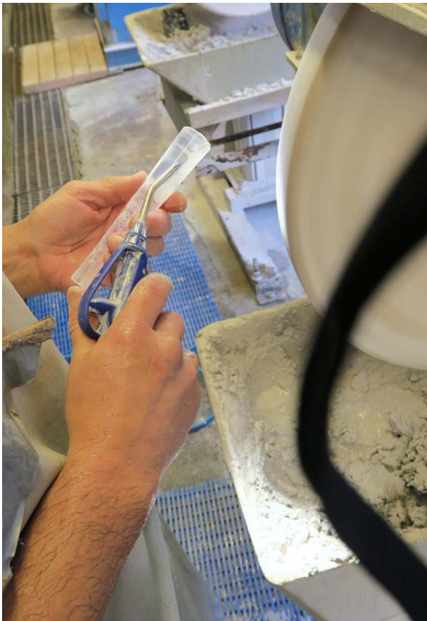
Anders shows how polishing is done with a synthetic polishing wheel.
