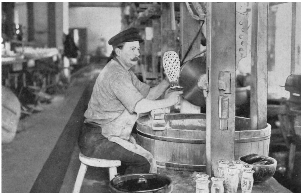
The grinder at his workplace, the early 1900s. The location where the photograph was taken is unknown. Next to the grinder is the rinsing bath. Illustration from Glaset förr och nu , Seitz, 1933.
