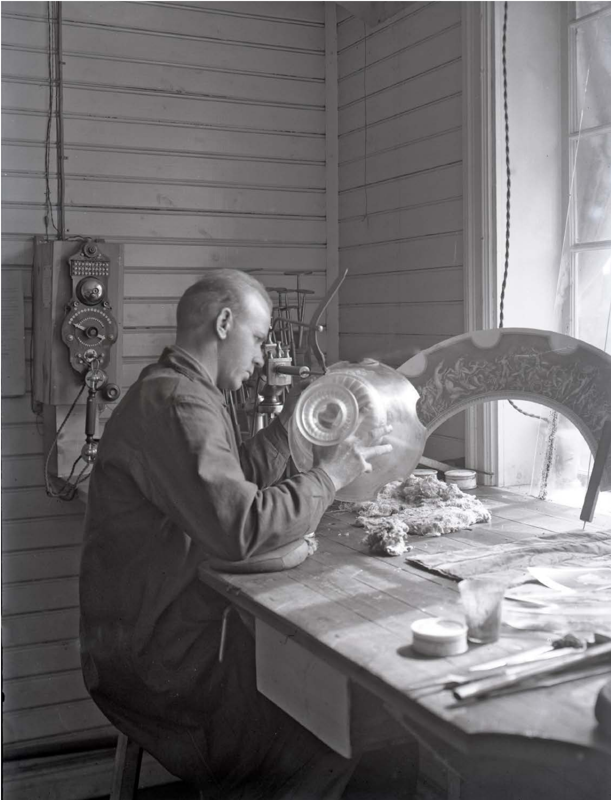
Before the Paris Exhibition in 1925, Gustav Abels was commissioned to engrave Simon Gate's Bacchus' Train. In front of the window is Gate's cardboard, the model Gustav had to copy from. In the foreground are containers with emery paste. The engraving took about 300 hours to perform and afterwards Gustav said that it was his most demanding job as an engraver. Photo: Winell, KLM archive.
