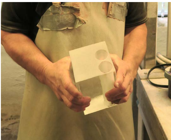
The glass block from which the blank for the handle has been drilled.
