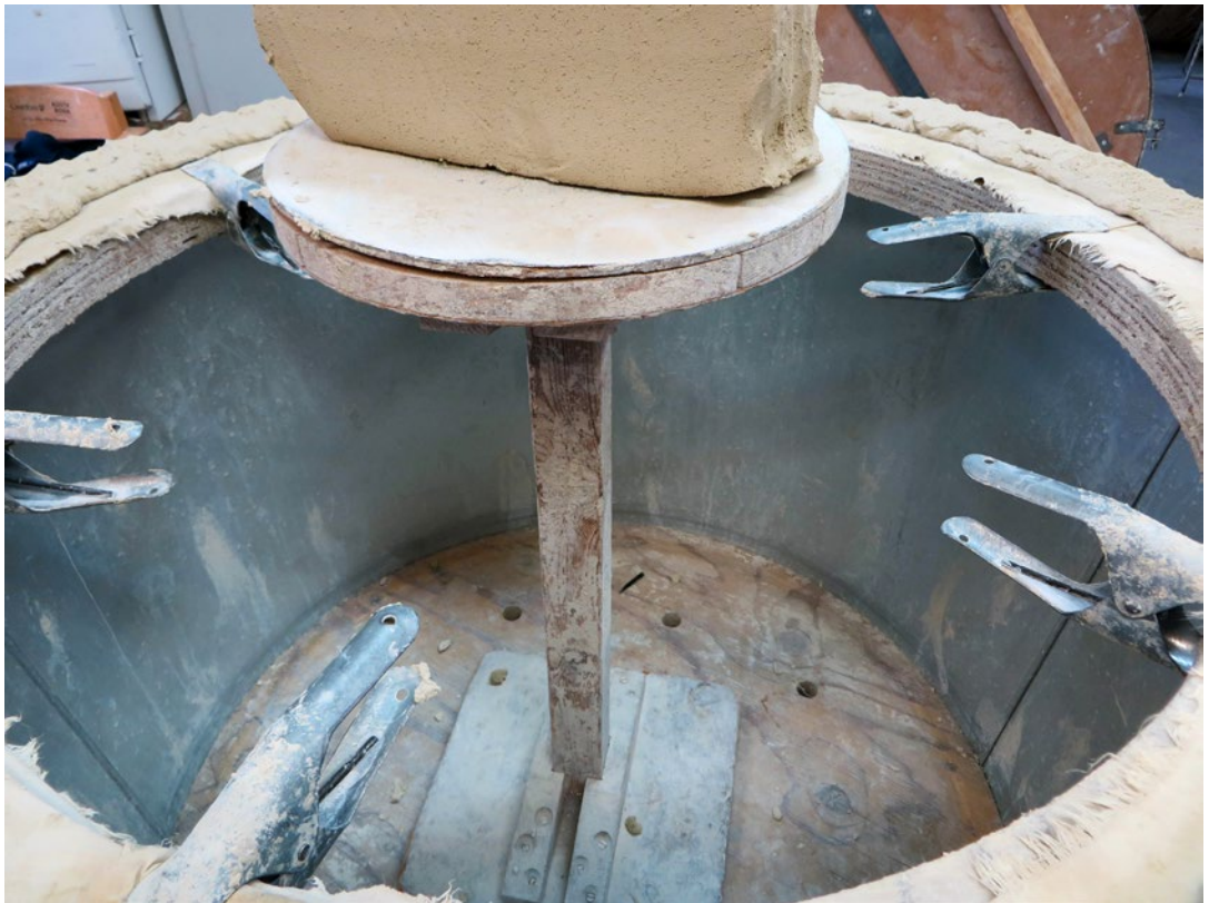
The sheet metal template is removed when the ten layers of the crucible are finished.
