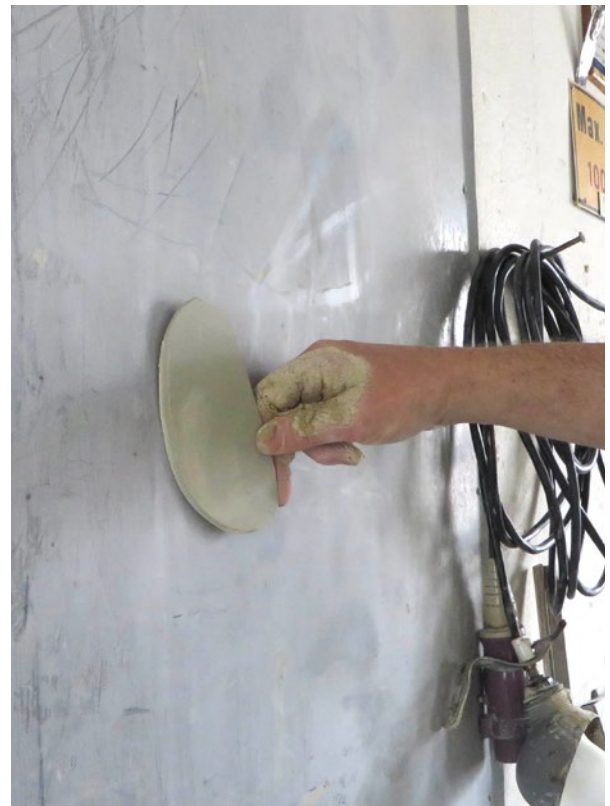
Different templates are used as guidelines to get the desired dimensions, which vary between different glass factories. A dimension is drawn on the wall.
