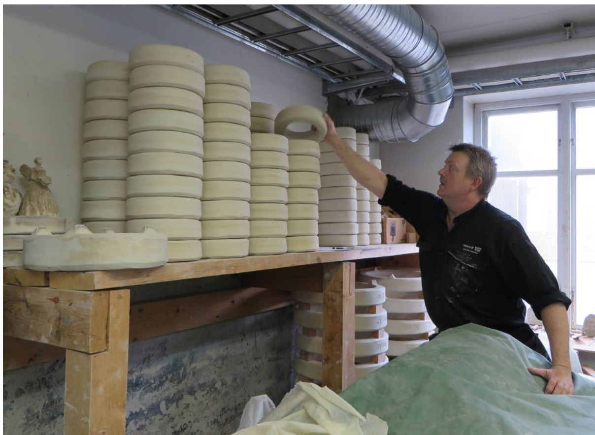
Various types of rings that will lie and float on the molten glass are also manufactured in the crucible workshop. This clay does not need to rest for long, and can be made from the first cast.
