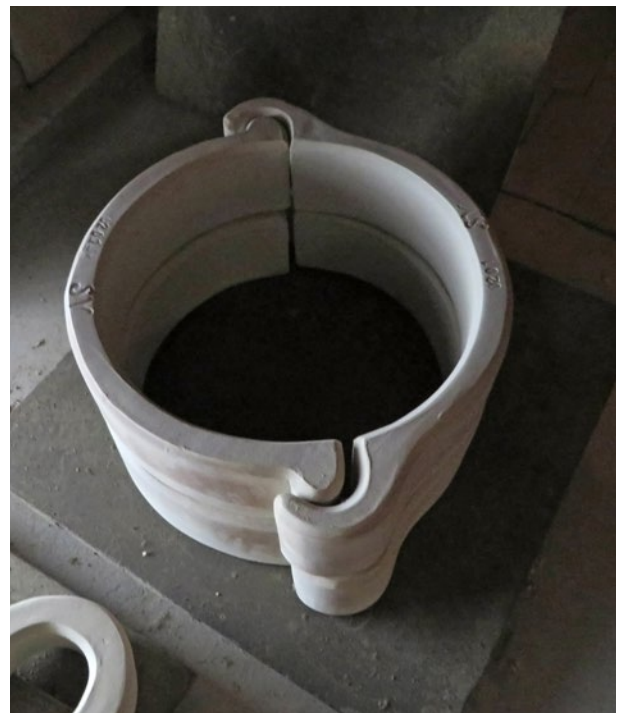
An openable ring is easier to put in the crucible but does not work as well.
