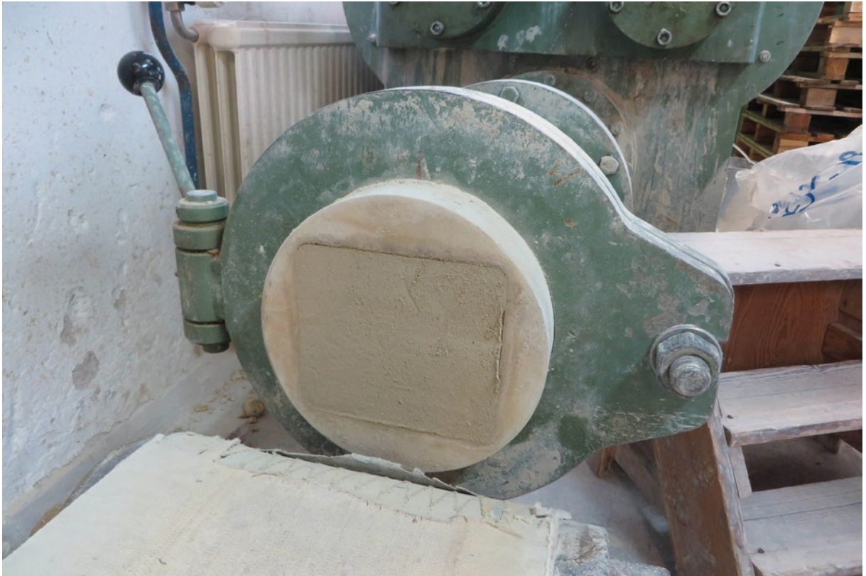
Clay extruder. The clay is pushed out in square lengths, which are stored on pallets in so-called casts.
