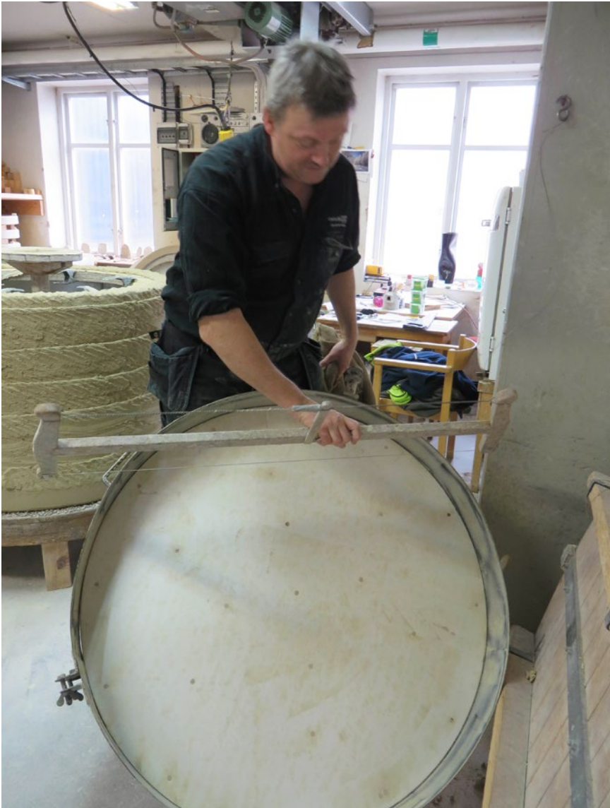
Peter Meinking shows how the wire saw is used when the base is finished.
