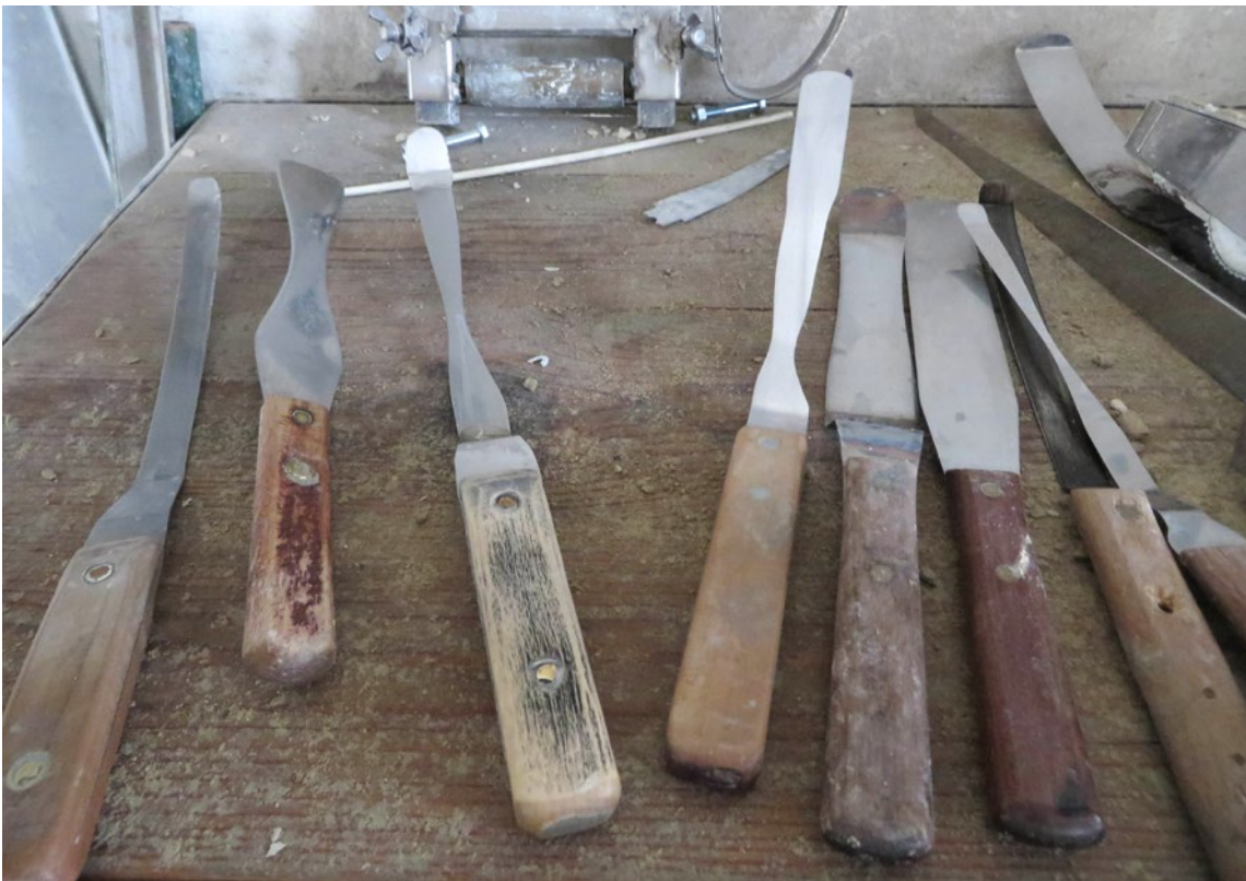
A knife, or most preferably "grandmother's old pancake spatula" in Swedish steel, is used to polish the outside and prick cavities. After several years of use, the spatulas are characteristically worn down.
