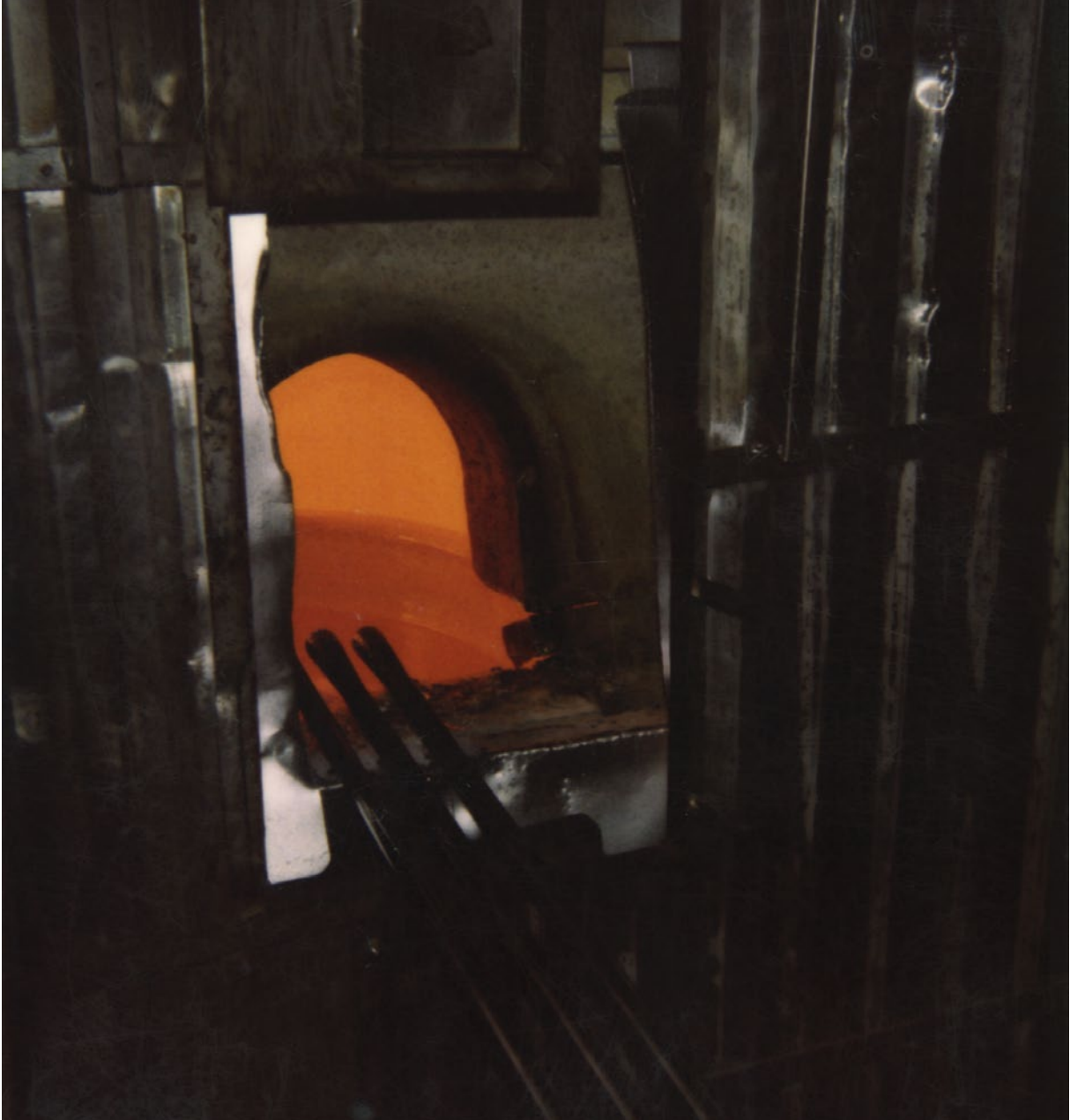
The crucible is subjected to great stress within the glass oven, where the glass mass can be heated to almost 1500 degrees Celsius. Photo: Peter Meinking/Per-Eric Deckert.
