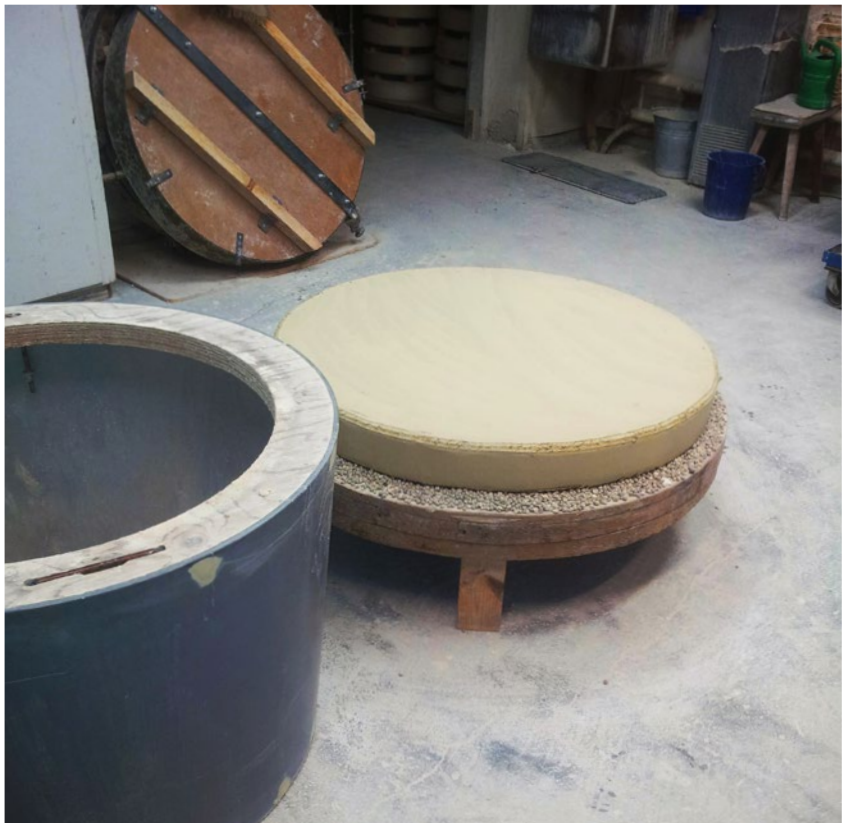
The finished base is turned upside down on a bed of gravel. Photo: Peter Meinking.
