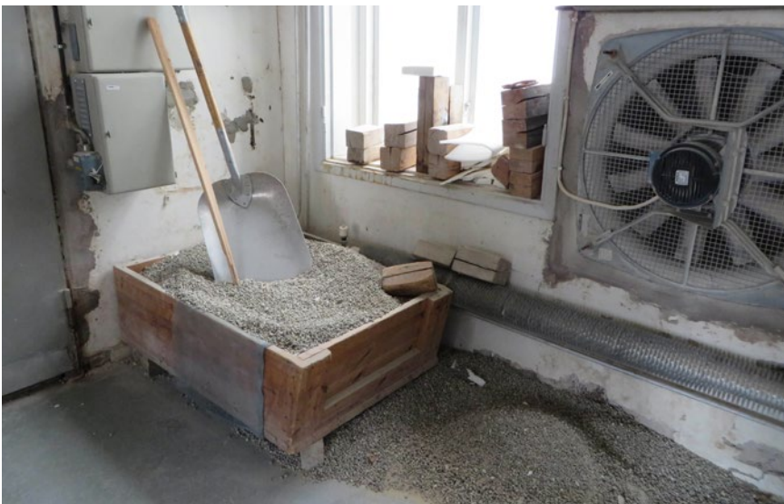
Gravel is used under the crucibles so that they do not get stuck.
