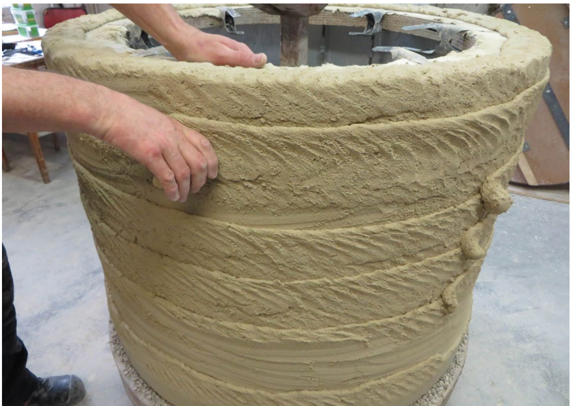
Peter Meinking shows how a piece of clay from the clump in the centre is used. The clay is on a pedestal in the middle to be close at hand. The clay is struck and pressed into the wall of the crucible, according to an English method.
