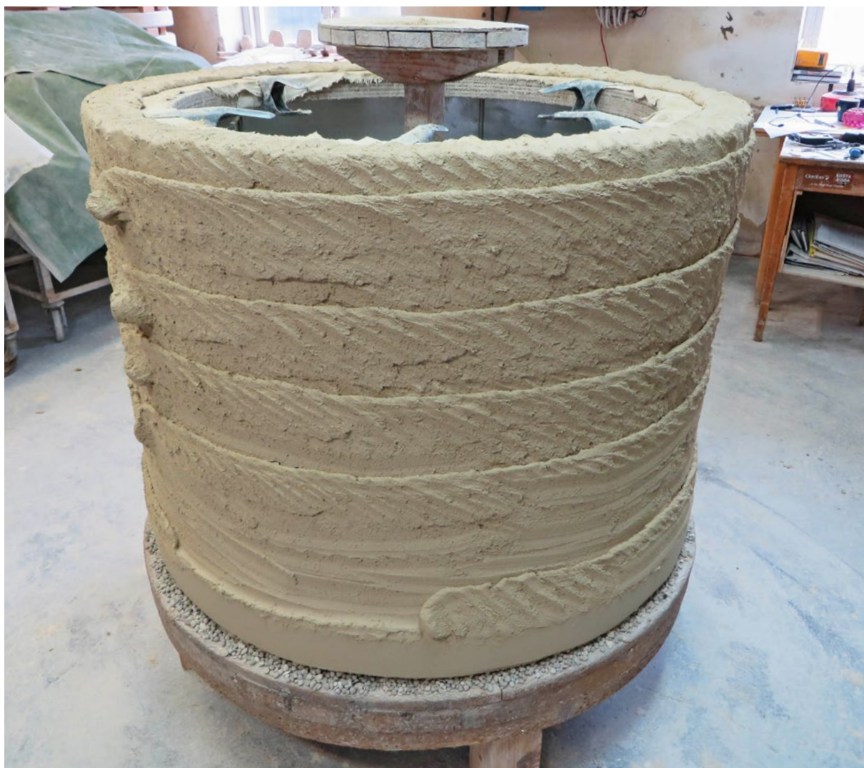
The crucible is "thumbed" by hand in 10 layers, according to the English method taught here by an Englishman, Mr Totel, 1947. The work has to be done in one go and takes 9 hours for a single man.
