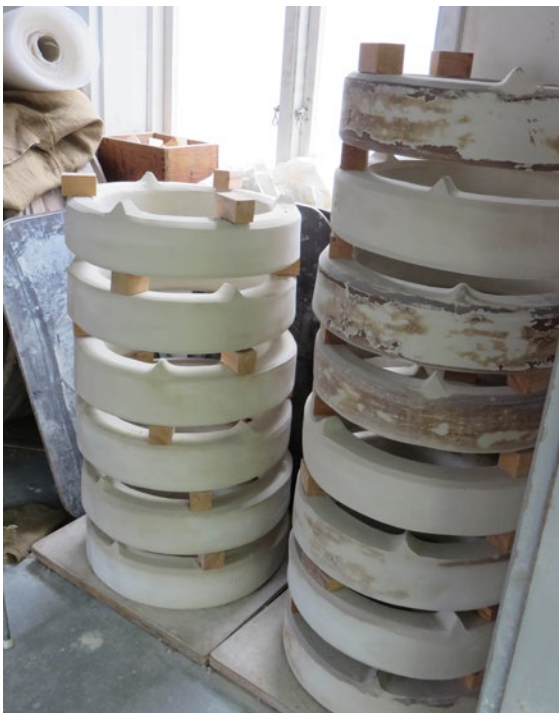
The rings do not need to rest in the humidity chamber but can dry directly in the crucible chamber before being allowed to rest in the attic alongside the crucibles.
