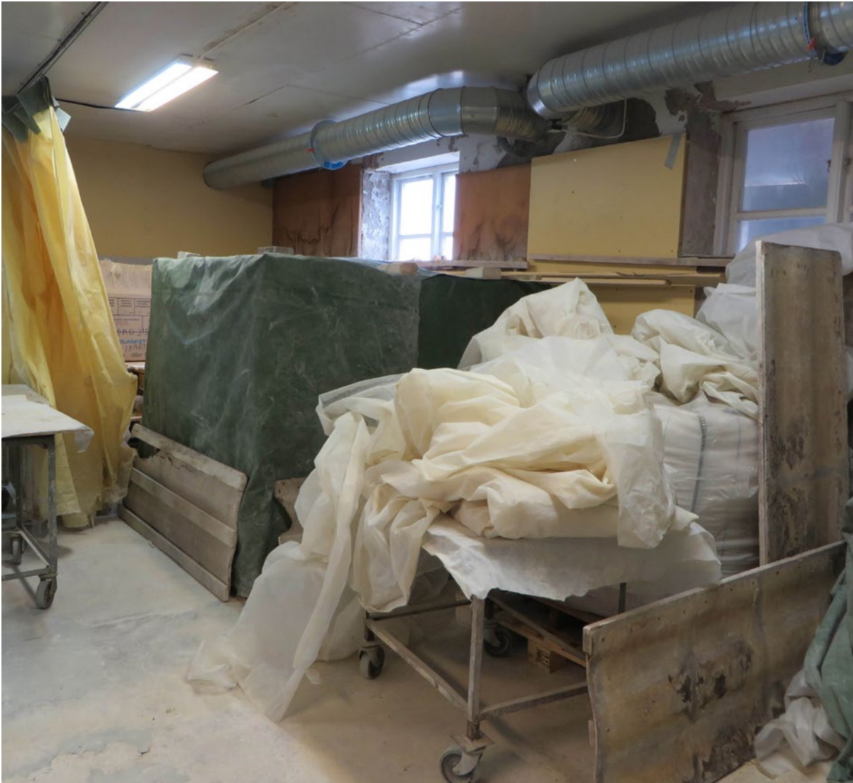
Four casts with clay lie under plastic against the outer wall to mature. In total, these rest at least eight weeks but usually more, sometimes for several years.
